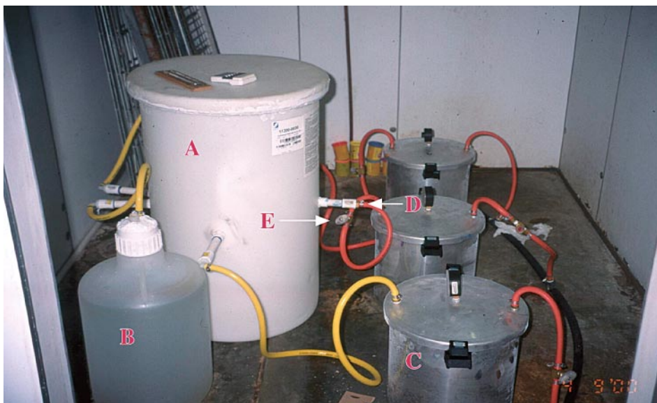
FIG. 1. Low-pressure storage (LPS). (A – filter; B – inlet of humidifier air; C – storage chamber; D – pressure gauge; E – valve regulator).
